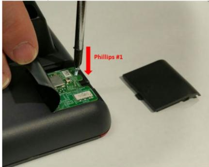
4. Use the Phillips #1 screwdriver to fasten the module.
