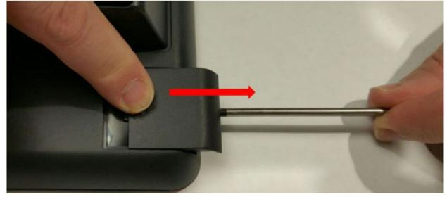
2. To remove the module panel, slide the panel out in the direction of the arrow.
