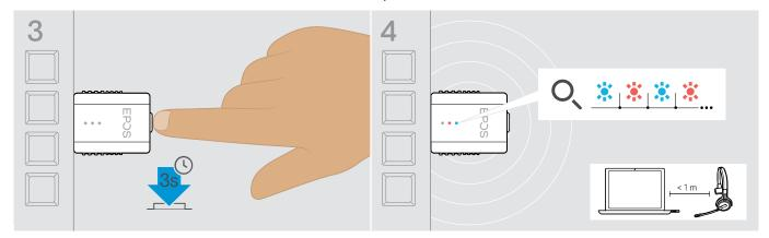
Press and hold the dongle's button for 3 seconds to enter pairing mode. The LED alternately flashes blue and red.
