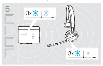
If pairing is successful, the dongle LED lights up dimmed blue and the headset LED switches off.
